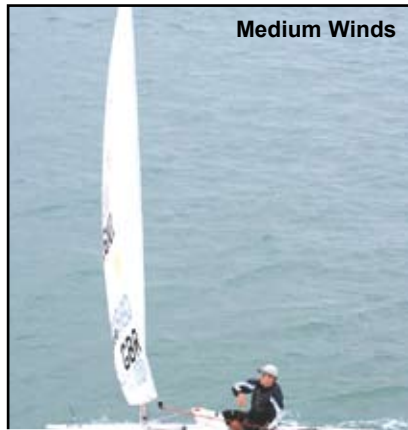
Note the boom is not at 90° but the top of the sail is due to the twist.
